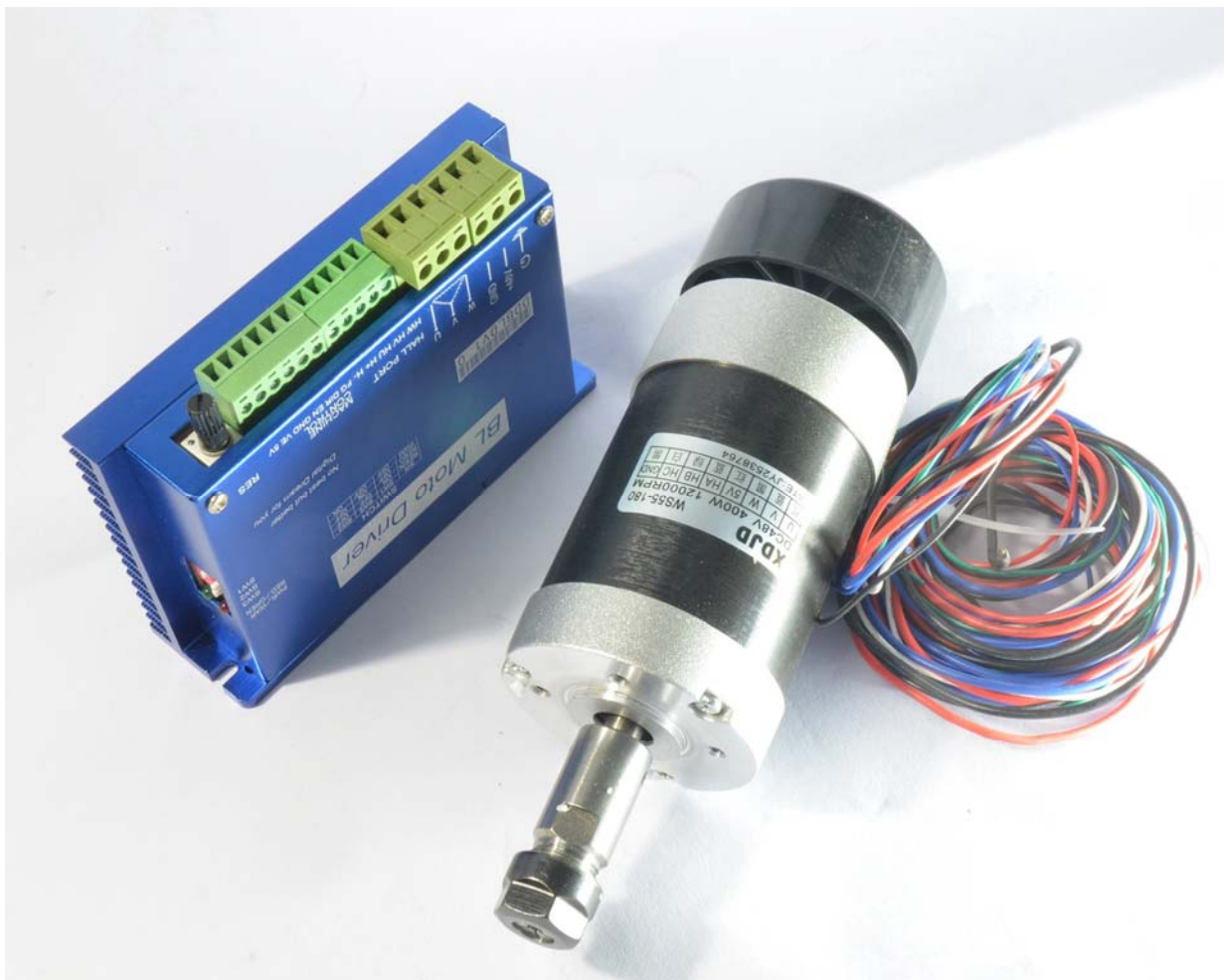
work in with 400W 12000r/min BL DC motor
