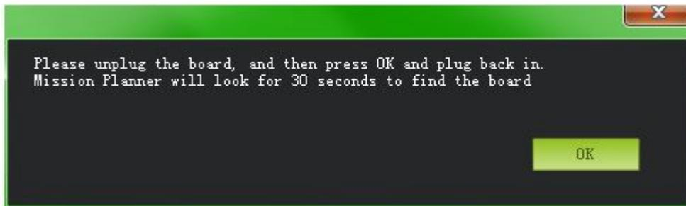
You need to disconnect the USB, and then click "OK" button, and after 30 seconds, you replug in the USB. This period of interval is for the Pixhawk to be prepared for firmware updating.
