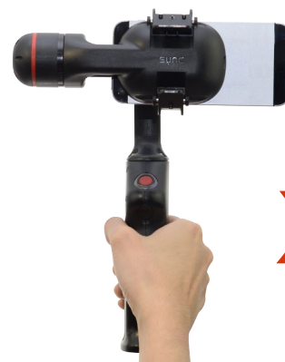
Wrong Pitch-axis motor direction
