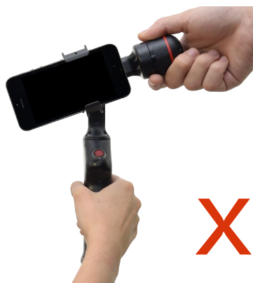
Wrong Pitch-axis motor direction
