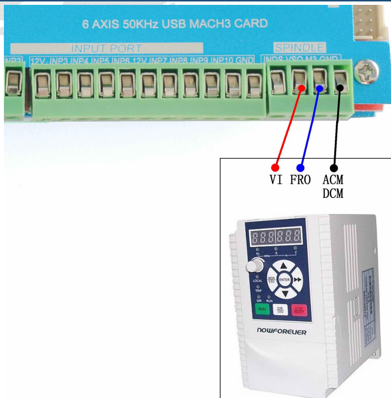
Figure2-7. spindle control output and inverter connection
