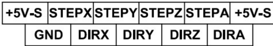
Picture 2-8. stepper/servo control output interface definition picture
