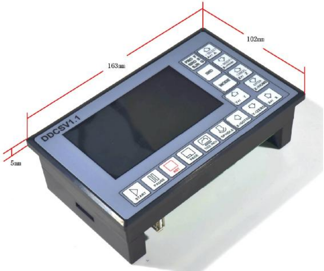
Picture1-1 DDCSV1.1Front external view and dimension figure
