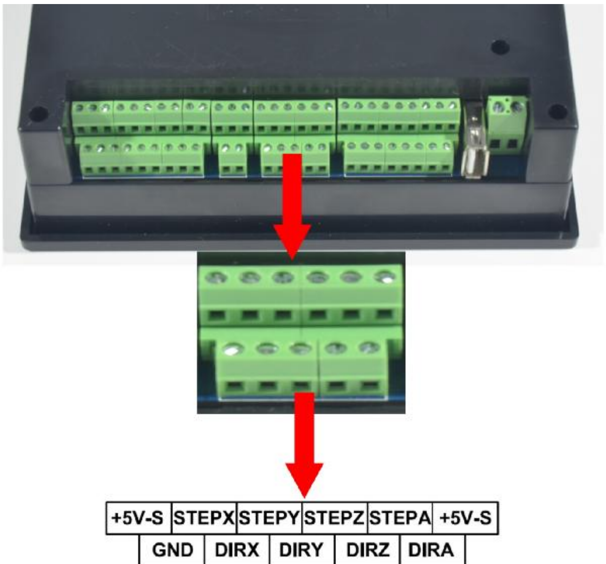
Picture 2-7. Product photo of stepper/servo control output wiring
