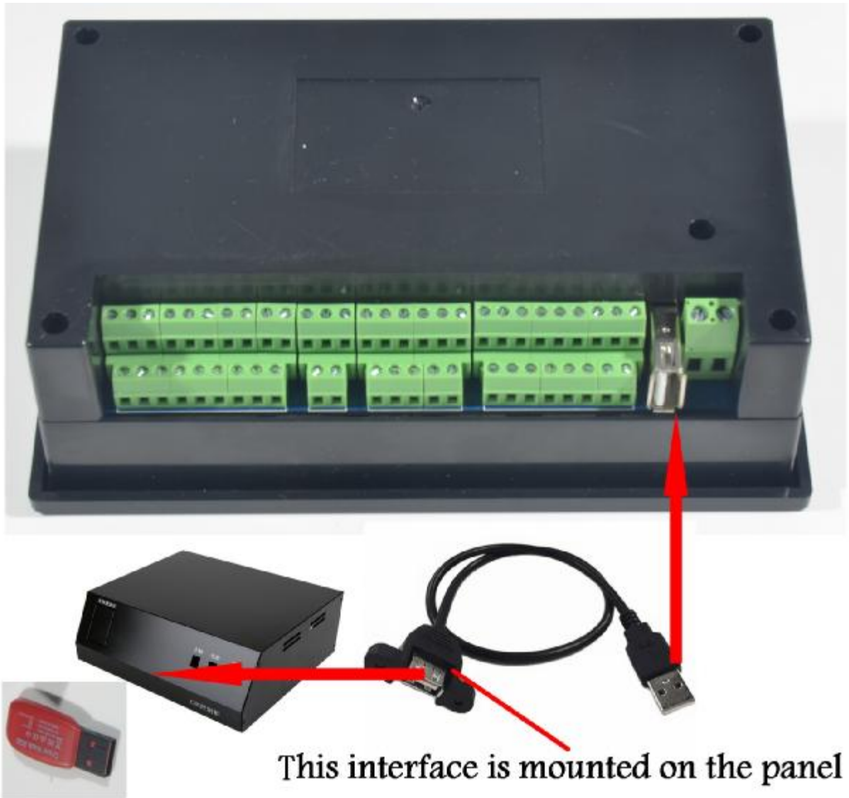
Picture 2-4. Sketch diagram of USB interface extension cord USB
