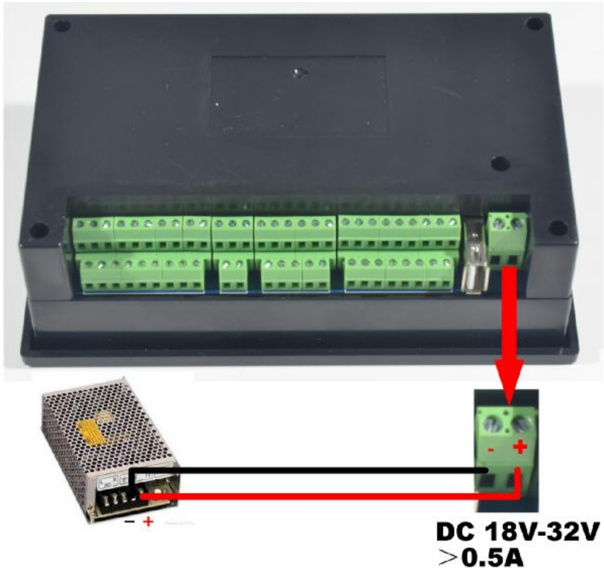
Picture 2-3. Main power input interface definition diagram
