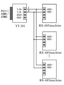
3.YT-30 half-duplex communication connect between interface converter
