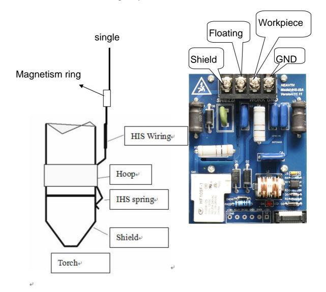
Working process: After the height controller receives the arc-on signal which is sent out from NC system, the cutting torch will fall down immediately. When the protector get to the material, the height controller will receive this signal, and then control the cutting torch to rise to the given Height of IHS. The height controller will control the plasma to arc on after IHS.
