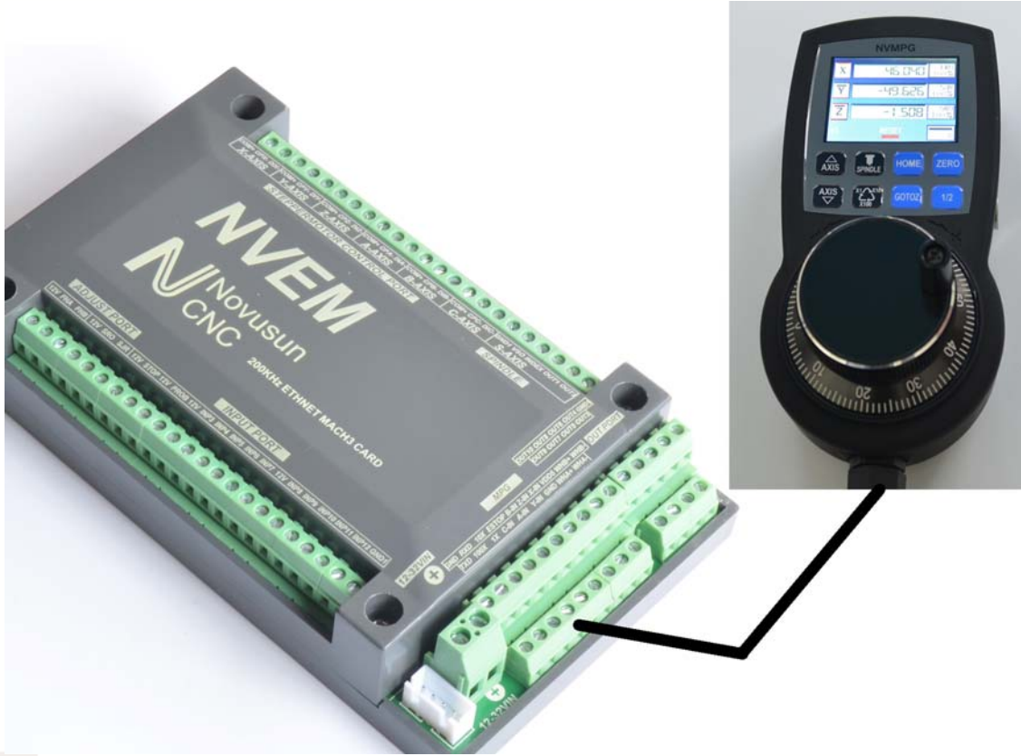
Figure 2-3 NVMPG connect to NVEM
