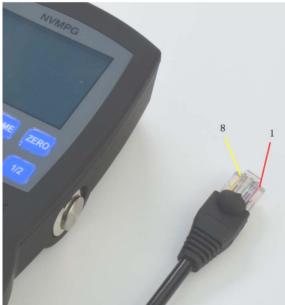
Figure2-2. Wire mark of NVMPG in RJ45 port mode
