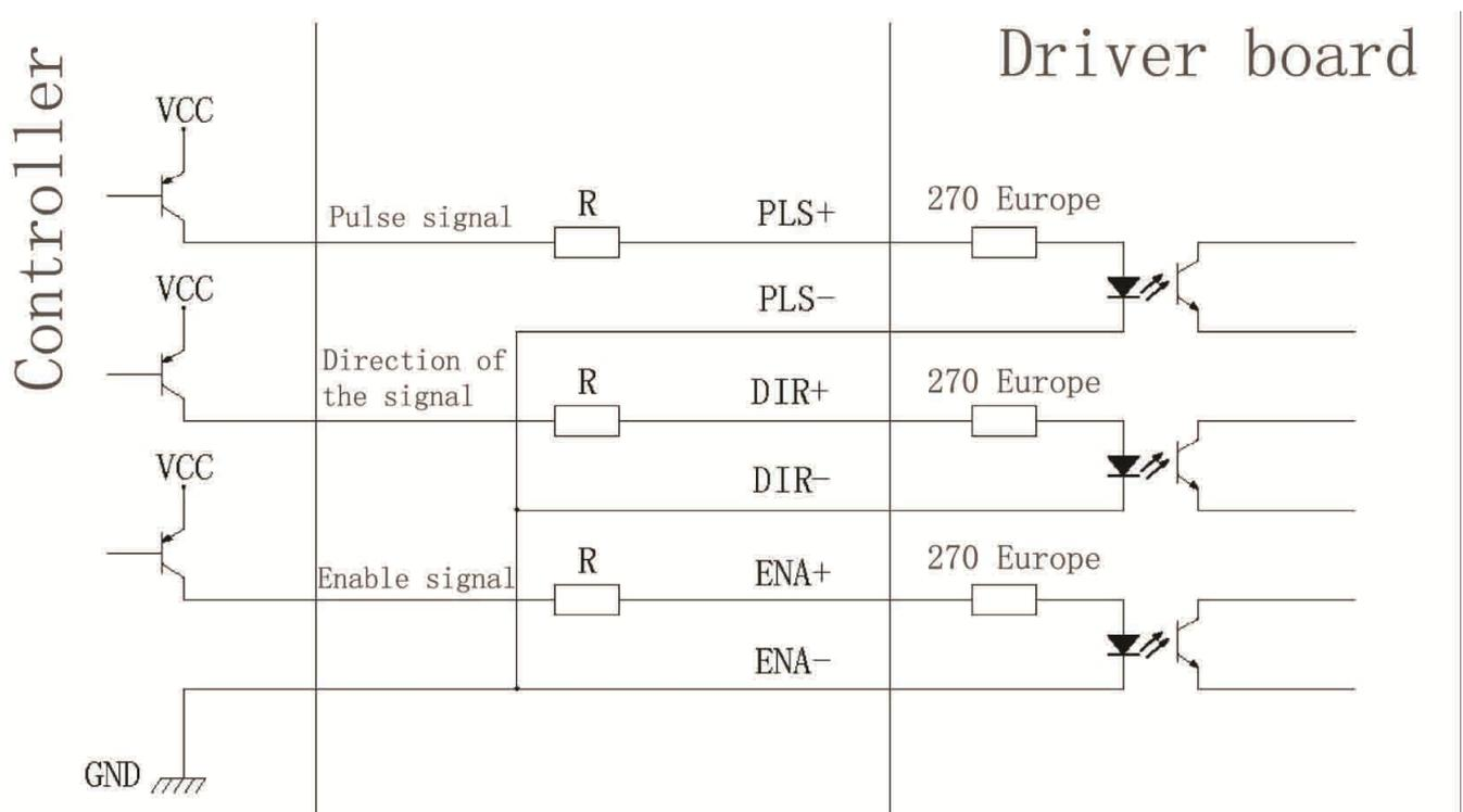
Figure 2. Input interface circuit (common cathode connection)
