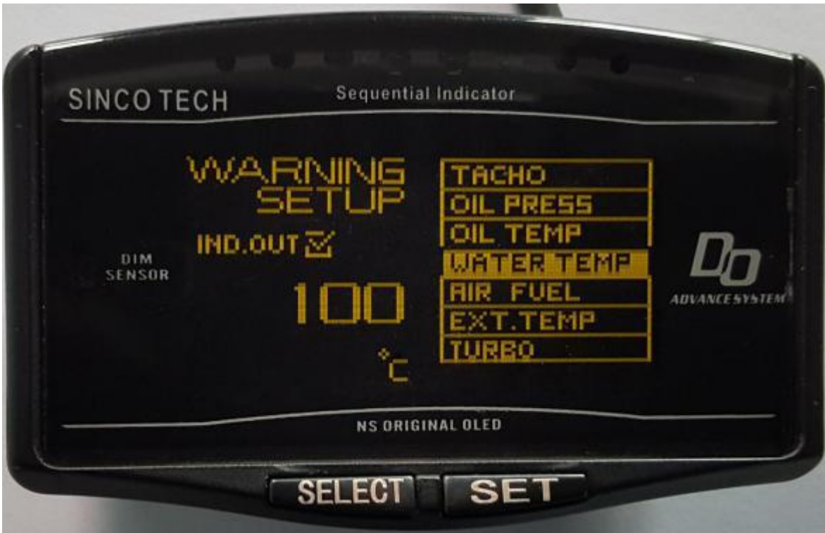
(5) WATER TEMP---set the water temperature value for alarm.
