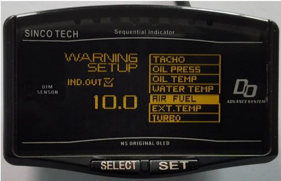
(6)AIR FUEL---set the air/fuel ratio for alarm.
