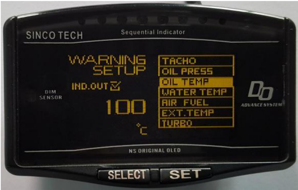
(4) OIL TEMP---set the oil temperature value for alarm.
