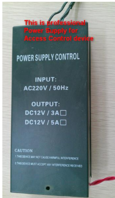
Figure 1: picture of access control power supply
